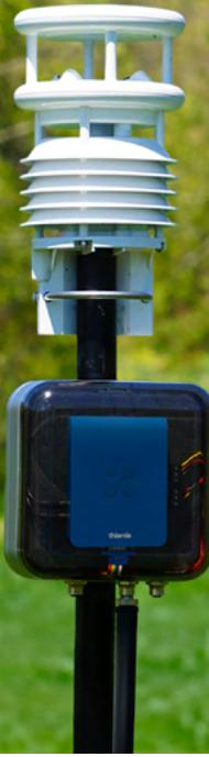
**Thiamis is a plug-and-play environmental monitoring platform trusted for over a decade and built for seamless integration with third-party sensors.** It combines system control, data logging, digital processing, GPS, and telemetry in a single device, and eliminates manual data retrieval by securely transmitting data over cellular or Wi-Fi to the Aethair Cloud for real-time access and analysis.
